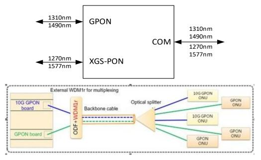
In the evolution to 10G GPON through co-existence, multiplexers must be deployed and fiber paths in CO equipment rooms must be reconstructed. This requires a high amount of effort. Is there any innovative product or solution available that reduces the effort and lowers cost?
