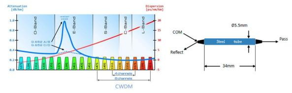
Like DWDM filters, the Red Blue filter is a thin-film filter device. It is a three-port device. One port is called the "COM" port, The other two ports provide the conduit for the two wavelength "bands." The two bands are the Blue ( $\lambda$  1530 to 1543nm) and the Red ( $\lambda$  1547 to 1561 nm). One band goes thru the Reflected port, and the other band goes thru the Pass port.
